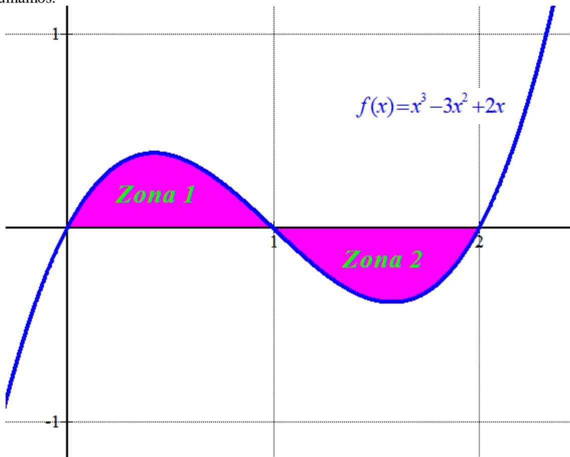
$$\text{Área 1} = \int_0^1 f(x) dx = \int_0^1 x^3 - 3x^2 + 2x dx = \left[ \frac{x^4}{4} - x^3 + x^2 \right]_0^1 =$$
